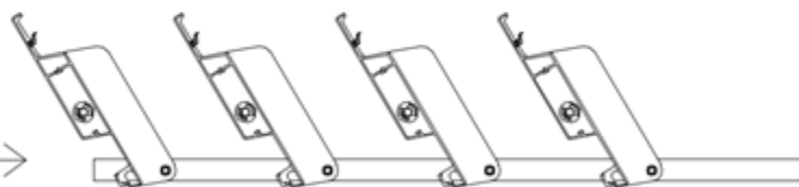
Fig. 2. Standard setting of blade opening direction in Pergola SB350
